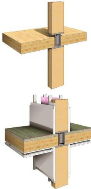
In the 10 story Brock Commons mass timber building (design: Acton Ostry) an encapsulation strategy was chosen to meet the 120 min fire resistance requirements (01).
